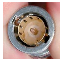
Neutrik BNC: no tilting due to side pull
